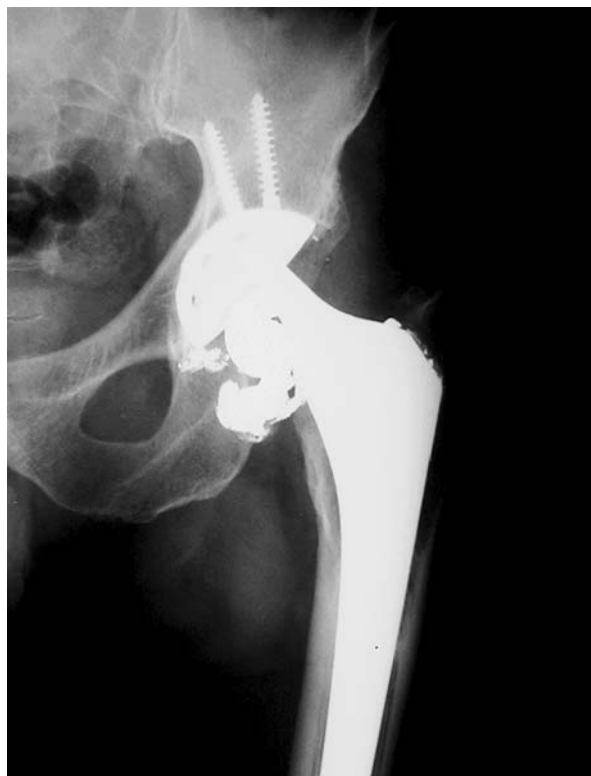
Figure 1 XR showing the evidence of the ball head fracture. The Y-TZP ball head fractured after 36 months, in atraumatic conditions.
